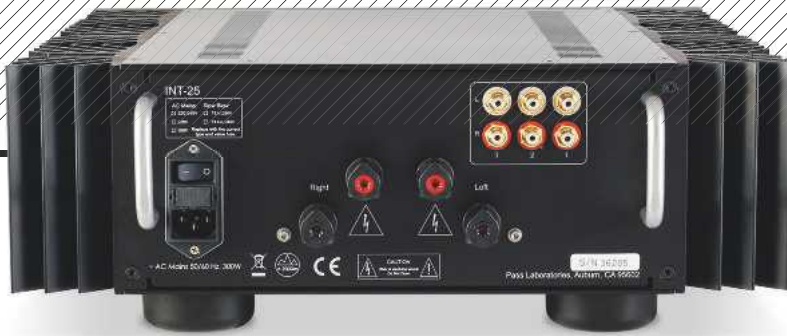
ABOVE: As simple as it gets – just three single-ended line inputs on RCAs and substantial 4mm speaker cable binding posts. The handles are largely decorative!
