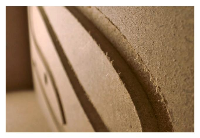
CGD involves routing a continuously curving groove, almost half-an-inch wide, that snakes down the cabinet wall. The groove is then filled with a rubbery compound, which helps reduce resonances. But that's not all there is to it—the constantly varying distances from the edges of the groove to the edges of the cabinet wall diminish resonances as well.
