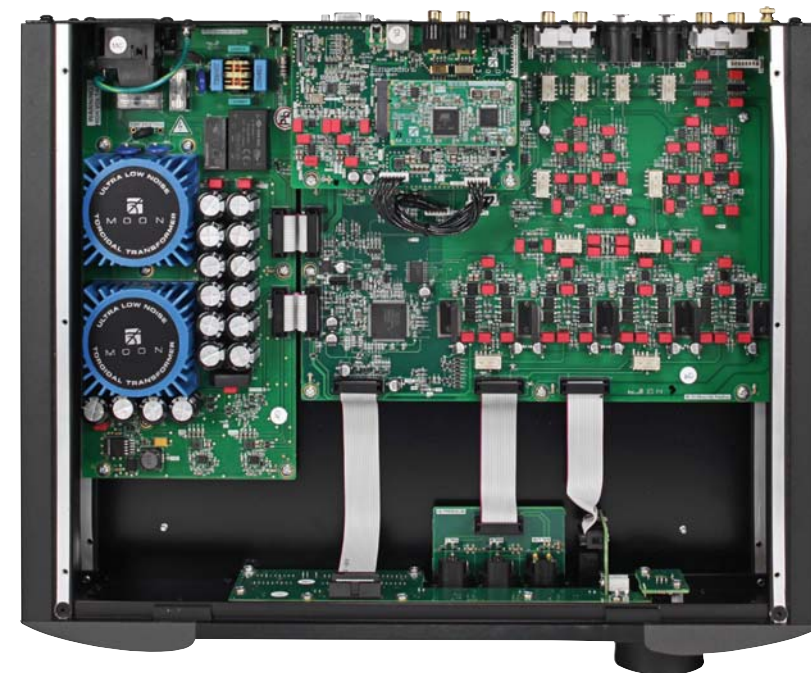
Twin toroidal transformers give the Moon Neo power to drive even the most insensitive of headphones.
