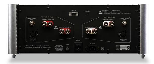
The rear panel boasts more connectors than are found on most power amps. Most noticeable are the four pairs of WBT binding posts -- two pairs per channel -- to ease biwiring. There are also pairs of single-ended and balanced inputs (I used the balanced throughout my listening), a nine-pin RS-232 port, a 12V trigger input and corresponding output, a fuse socket, an IEC-compatible power-cord inlet, and, finally, a rocker switch to turn the mains power to the amplifier on and off.
