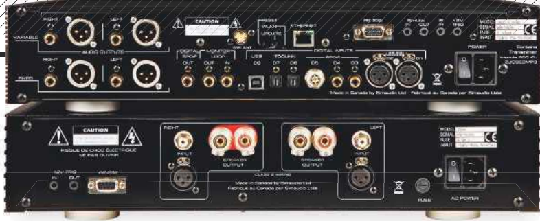
ABOVE: With eight digital inputs of all varieties – and the network client providing a ninth digital source – both single-ended (RCA) and balanced (XLR) analogue outputs are provided. Power amp has balanced inputs too, plus RS-232 and 12V triggers
