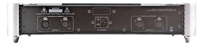
The rear panel is where all the action is. There are two sets of outputs labeled Analog and two sets labeled Digital. Outputs are on XLR like barrel connectors, the Analog connections having four pins and the Digital connections having five. There is no way to plug them in wrong. Output voltages are listed as +/- 20 V for Analog and +14 V for Digital. Two full sets of connecting cables come with the unit. They
