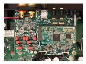
The first step is replacing the D2 board. To do that, you pop off the amp's top cover, remove the screws that attach the old DAC board to the amplifier's main circuit board, remove the two jumper cables connecting the DAC and main board, and remove the screws attaching the DAC's jack panel to the amplifier's rear plate. Then reverse the process to install the D3 board.
