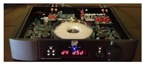
The new D3 board allows this. Employing the ES9018K2M Sabre32 Reference DAC chip from ESS Technology, it supports native DSD playback (up to quad-rate: DSD 256), and PCM to 32 bits/384kHz, over USB.
