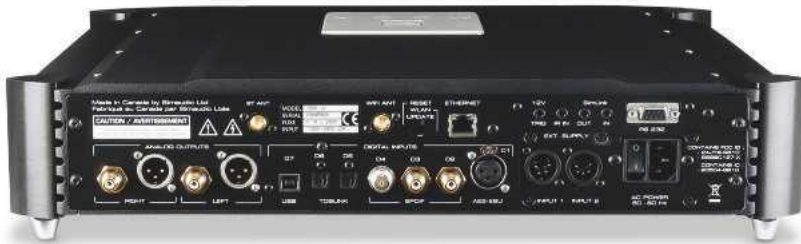
ABOVE: Wired and wireless network inputs (and a BT antenna) join another seven digital inputs – USB-B, three coax and two optical S/PDIF, plus AES/EBU. Single-ended and balanced outputs on RCA/XLRs are joined by ext. PSU inputs and 3.5mm triggers
