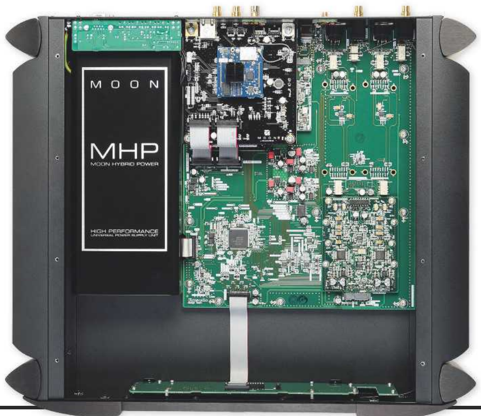
RIGHT: Screened PSU [left] feeds 12 separately regulated supplies for the Stream 810 Wi-Fi board [blue], the network adapter [brown, underneath] and main audio board with its pair of ES9018S DACs [daughter PCB, right]
