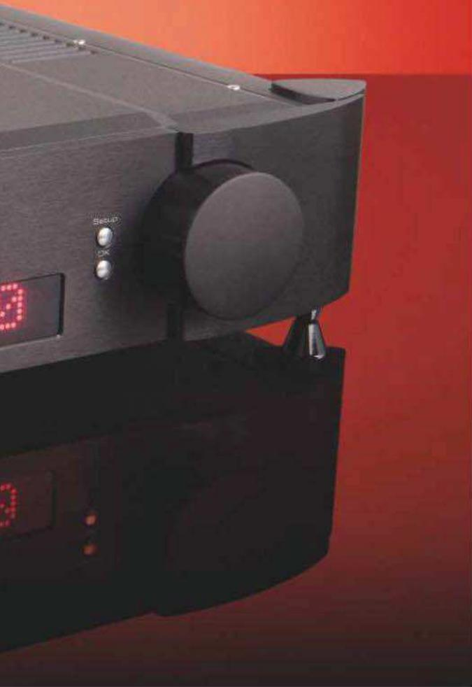
entirely should you so wish. All this is accessible via the front panel's Setup button, sitting just to the left of the main volume control. The main display is a large dot-matrix-style red LED affair, and is striking and easily readable from a distance. It's defeatable should you so wish. Other minor controls include input and balance, mute and standby. All of this is duplicated on the supplied, and rather swish remote control.
