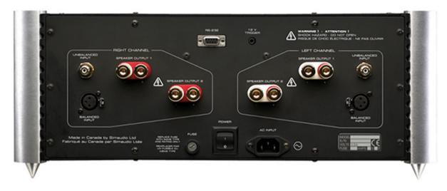
The main power switch is at the rear panel, if you want to use the single-ended inputs you need to use supplied jumpers for XLR inputs pins. The 870A provides two pairs of speaker terminals to make bi-wiring easier.
