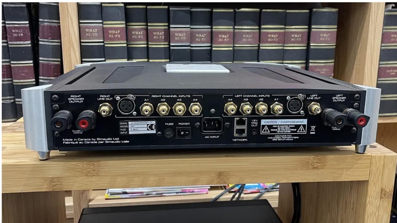
If you are expecting the full bells and whistles approach from the collection's only integrated amplifier then the 641 is going to disappoint you. This is purely a line-level device with no digital inputs, phono stage or headphone output. Bluetooth? Not on the menu either, which is a bit of a shame considering the way it would open up this amplifier for use across a wider range of sources.
