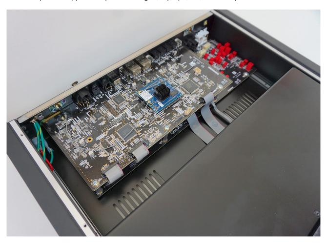
Noise can still get into the unit which is why the generation of analogue, linear power supplies, mentioned above, is performed. That, "...effectively prevents noise getting into the unit."
