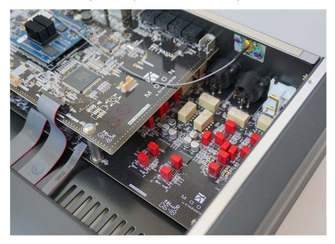
All of the digital inputs on the rear run to 32bit/384kHz and DSD256 via an ESS DAC PRO chipset. USB is full asynchronous. There's also a USB host socket to attach a thumb drive. The content information for that drive is then listed on the app – a nice touch. There's also a healthy supply (four) of HDMI inputs for Smart TV and Blu-ray use. This turns the 390 into a 2-channel AV amplifier. The HDMI sockets are fully isolated and are 4K compatible.
