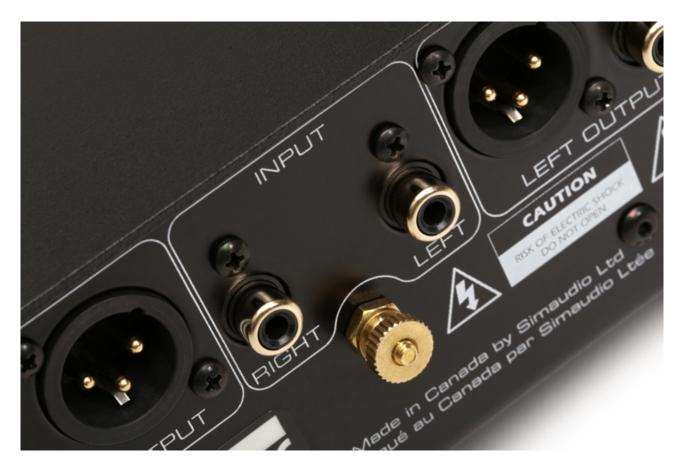
On the back of the unit there is a pair of single-ended RCA inputs, with a ground post located directly beneath them. Flanking them are single-ended RCA and balanced XLR outputs for the left and right
