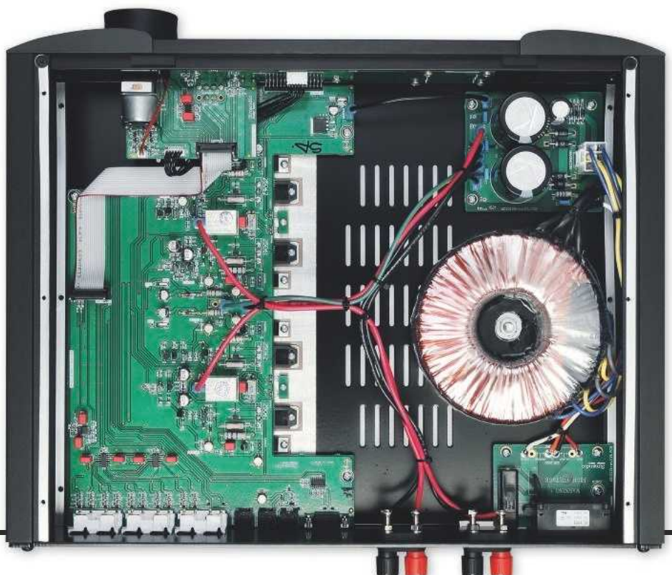
RIGHT: Once upon a time, every integrated amp looked like this! Large toroidal transformer [right] feeds regulated PSU [top right] for a fully discrete pre/power circuit with custom bipolar output devices [on centre heatsink]
