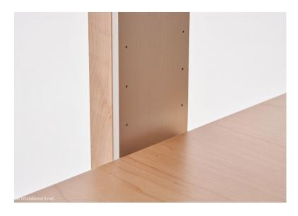
Thanks to the three-centimetre hole pattern in the side aluminum pillars, the height position of the levels can be adjusted to suit individual requirements. The T-profile is extremely rigid so that the side spikes that engage in the micro-hole grid can be tightened firmly. Despite the small distance between the two spikes, the levels are very stable against tilting.
