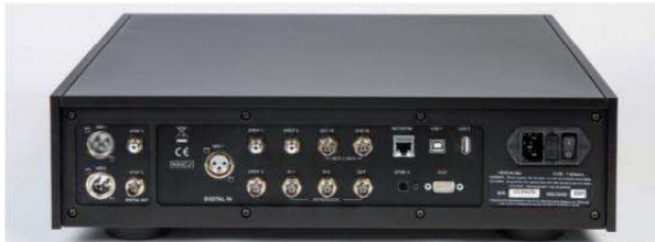
The Vivaldi Upsampler's rear panel includes an Ethernet jack for use with uPnP-based servers.
