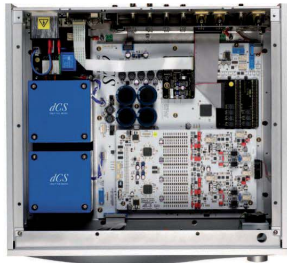
The Ring DAC’s array of latches can be seen in the center of the bottom board, with the two large FPGA chips to their left.
