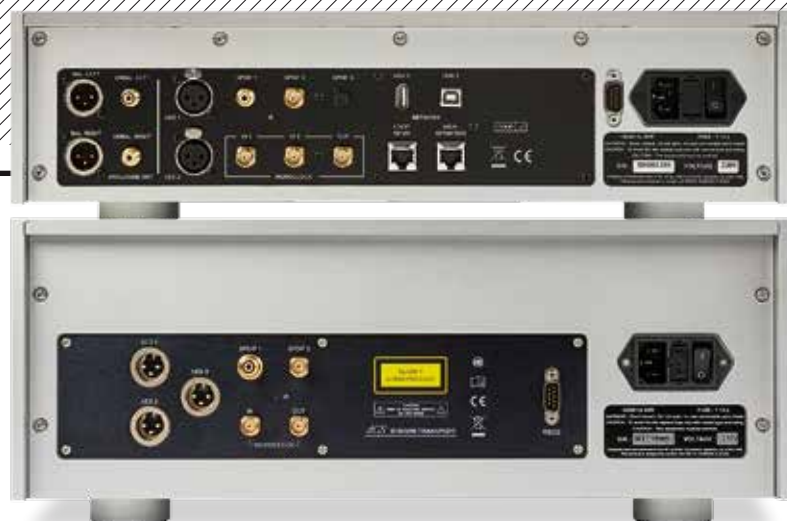
ABOVE: Transport [bottom] offers CD and downsampled SACD digital out on S/PDIF (coax and BNC) and AES (XLR). Upsampled DXD and native SACD is output on dual-AES connections. Clock in/out are mirrored on DAC [top] with three S/PDIF ins, one USB-B, USB-A, dual-AES and LAN plus single-ended (RCA) and balanced (XLR) analogue outs
