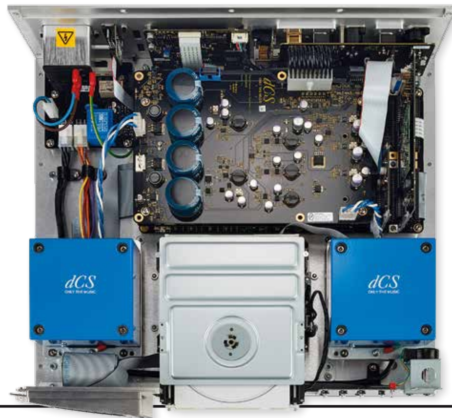
RIGHT: The dual laser CD/SACD mechanism [lower centre] features a 2mm steel frame, cast aluminium disc tray and is flanked by two screened PSU transformers [blue] feeding the transport and digital electronics
