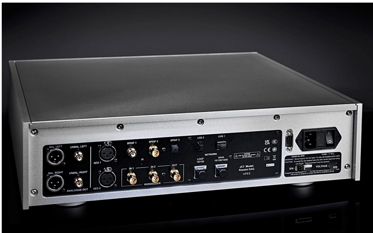
At the back, balanced and single-ended outputs; inputs 2 x AES/EBU on XLR, 1 x BNC, 1 x SPDIF on RCA and optical Toslink, USB A and B. Plus BNC in and out connectors for an external clock.
