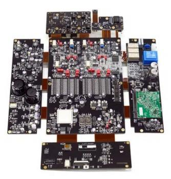
Lina Network DAC housing is far narrower than the Bartok yet it must accommodate essentially the same board. To that end, dCS essentially folded the board with key components on the sides of the housing with ribbon connectors rather than a more spatially demanding original flat design.
