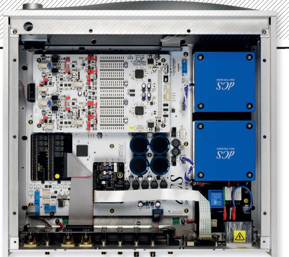
ABOVE: The 96 latches (a matrix of 2x48) that comprise the Ring DAC core are visible here with the two driving FPGAs sitting alongside [see boxout, p23]. The balanced analogue output lies to the left
