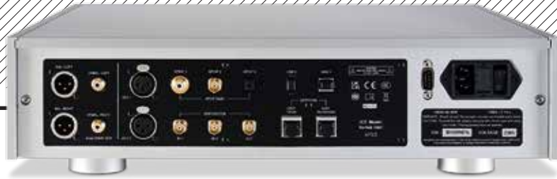
ABOVE: Digital inputs span S/PDIF (two coax, one opt), two AES/EBU (on XLRs), one USB-A for external HDDs, one USB-B for computer connection and a network port (on RJ45) – joined by clock I/Os (on BNCs) and variable analogue outs (RCA and XLR)
