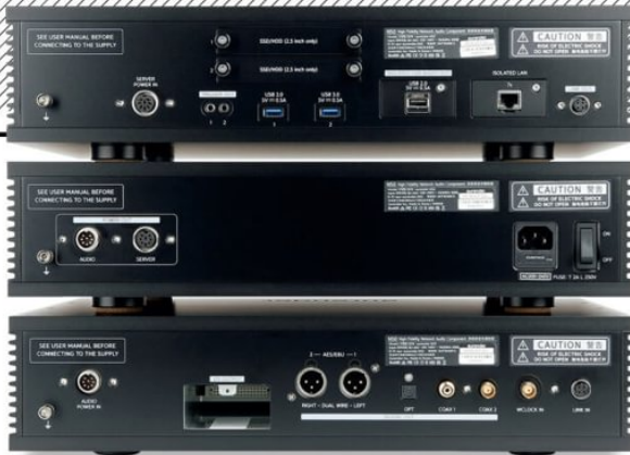
ABOVE: The N50 Server [top] includes two bays for 2.5in drives, two USB-A 3.0 ports for external media, an isolated Ethernet port and a filtered/isolated USB-A 2.0 'audio' output (to 1536kHz PCM/DSD1024). A proprietary data socket connects the Server with the 'Audio' unit [bottom], which offers alternate coax (x2), optical and dual-AES digital outs. The PS output module [bottom left] is removed in this picture
