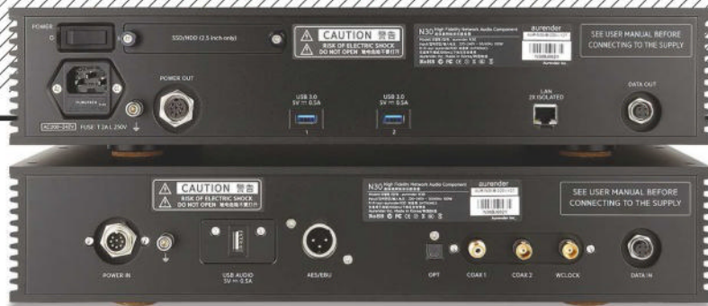
ABOVE: Two USB-A 3.0 hubs for outboard drives, a bay for a 2.5in SATA drive and a double-isolated Gigabit Ethernet port service the input/display chassis [top] which sends a PSU feed and digital data to the 'audio' chassis [bottom] with its outputs on USB-A 2.0 (384kHz/32-bit; DSD512) and AES/coaxial/optical (192kHz/24-bit)
