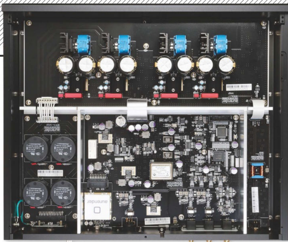
ABOVE: There's additional filtering [lower left] and choke-regulation of the incoming power supply [top] and galvanic isolation of the incoming data [lower right]. Within the screened 'audio board' there's an OCXO [centre], FPGA [top right] and custom USB audio module [lower left]
