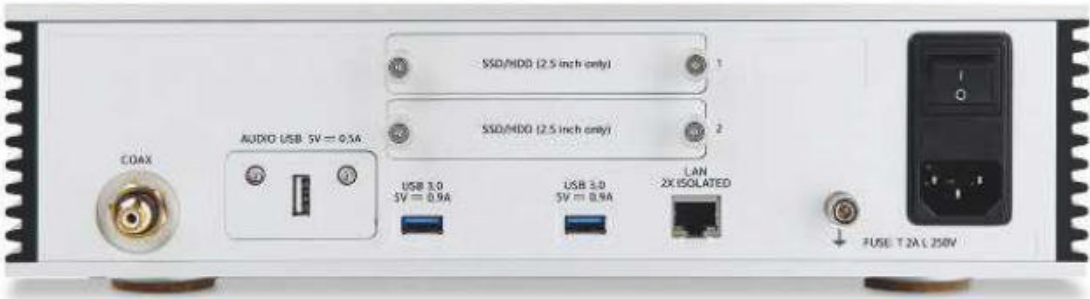
ABOVE: The N200 includes an isolated Gigabit Ethernet port, two USB-A 3.0 hubs for outboard drives, and two bays [above] for user-installed 2.5in SSDs or HDDs. Outputs are on USB-A 2.0 (to 384kHz/32-bit; DSD512) and coaxial S/PDIF (to 192kHz/24-bit)
