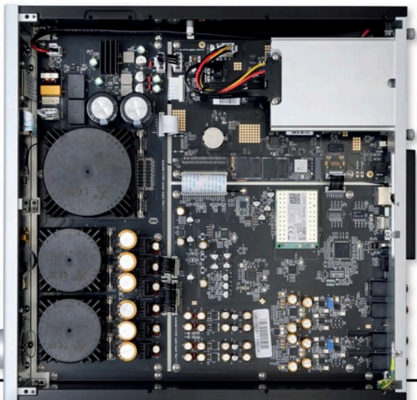
RIGHT: Multiple linear PSUs [left] power the Quad-core 2.0GHz CPU, 120GB NVMe cache and 2.5in drive bay [all top right] plus the audio PCB with two AK4490REQ DACs [bottom right] and Libre (Google Cast) network module [centre]
