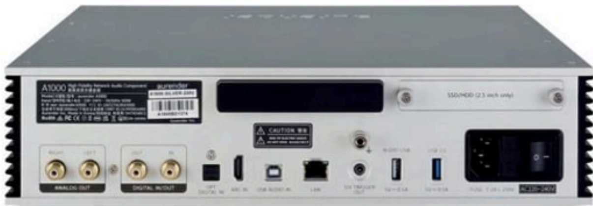
ABOVE: A USB-A host port for external drives joins a bay for one internal 2.5in drive, plus coax, opt, HDMI ARC, USB-B and Ethernet inputs and BT [black bar, top]. Digital outs are on coax and USB-A (768kHz/32-bit; DSD5 12) alongside analogue outs (RCAs)
