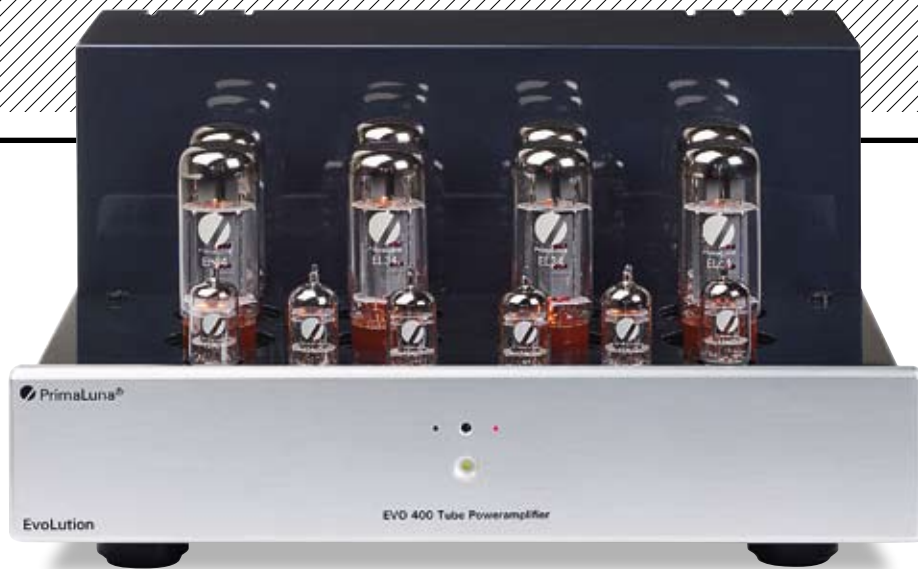
ABOVE: At 31kg, the EVO 400 power amp's bulk stems from the toroidal PSU transformer and two custom output transformers [all in screening can, behind]. Red LED on the fascia means the two pairs of EL34 pentodes (per channel) are configured in Ultralinear mode; green LED indicates triode mode
