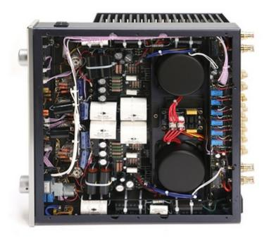
Removing the bottom cover is a visual feast for the geek/aficionado. A cursory look reveals an expensive **ALPS** volume pot, along with resistors and capacitors from Nichicon, Rubycon, Kemet, Takman, DuRoch, and others. This is the kind of stuff that one usually finds lurking in amplifiers costing 3-5 times as much.
