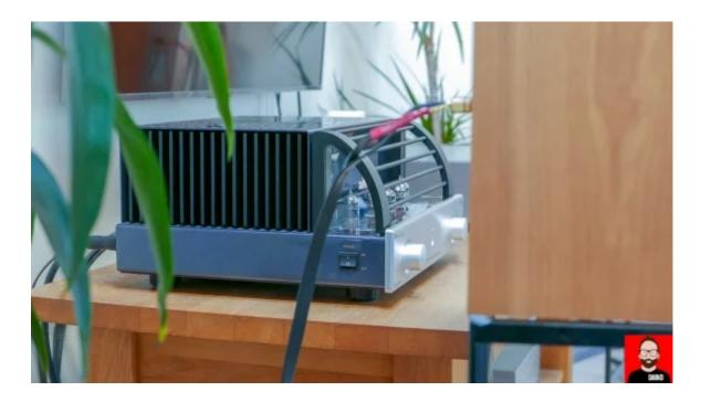
PrimaLuna is known primarily for valve amplifiers (aka tube amplifiers). The EVO 300 Hybrid is the company's first foray into hybrid electronics, marrying a valve pre-amplifier to a solid-state power amplifier. The preamplifier stage is based closely on the circuitry of PrimaLuna's Evo 300/400 preamplifiers, minus the tube rectification. That still leaves six 12AU7 valves to shepherd the signal to the power amplifier – the EVO 300 Hybrid has serious valve-preamplifier chops.
