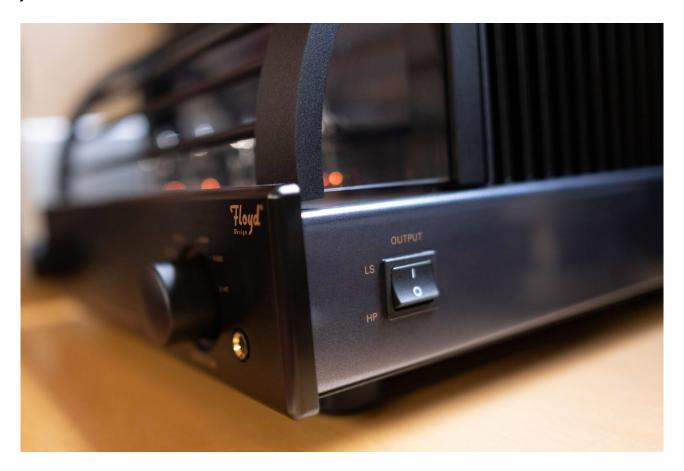
In a bit of a twist, a pair of switches reside on either side of the EVO 300—the switch on the left side powers on/off the EVO 300, while the switch on the right is for setting the output for speakers or the headphone amp. If you suddenly and unexpectedly find no music coming out of your speakers, make sure you didn't inadvertently hit that switch to its "HP" position. Not that I did, mind you (wink). The included aluminum remote is nearly heavy enough to be tactical. Nice.
