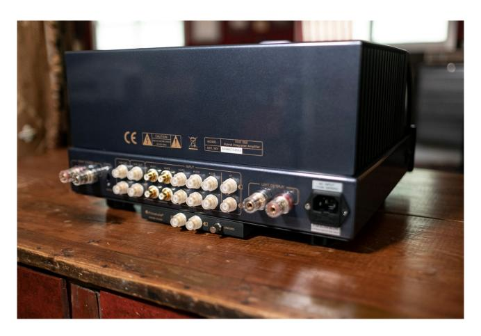
The EVO 300 offers 5 stereo RCA inputs, a stereo RCA Home Theater Bypass input, a single set of speaker binding posts, RCA Stereo/Mono Subwoofer out, Stereo RCA Tape Out, and a 1/4" Headphone jack mounted up front that is powered by the same internal amp as the speakers (look ma, no op-amps). There's also an optional belly-mounted MM phonostage, absent on the review sample (the case is there, the optional phono board isn't in it).
