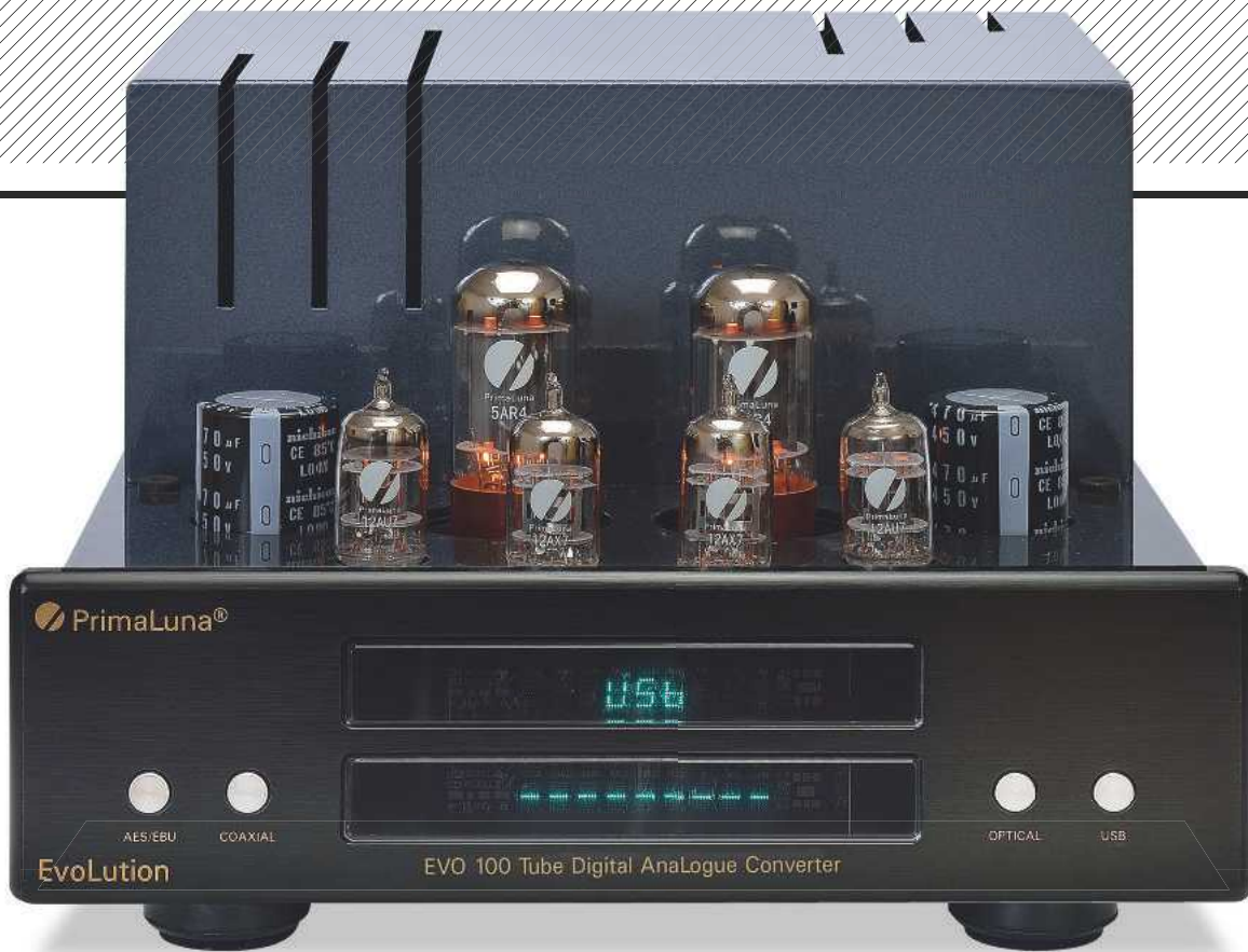
LEFT: Lifting the protective/decorative cage reveals a pair of 12AX7 and 12AU7 triodes in the audio circuit and two large 5AR4 tube rectifiers in the DAC's power supply. The selected input and sample rate is revealed in two displays, below
