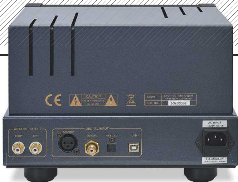
ABOVE: Simplicity itself – four standard digital inputs are fitted including AES/EBU (XLR), S/PDIF (on RCA and optical) and USB-B for computer connection. Fixed, transformer-coupled analogue outputs are on single-ended (RCA) connections only
