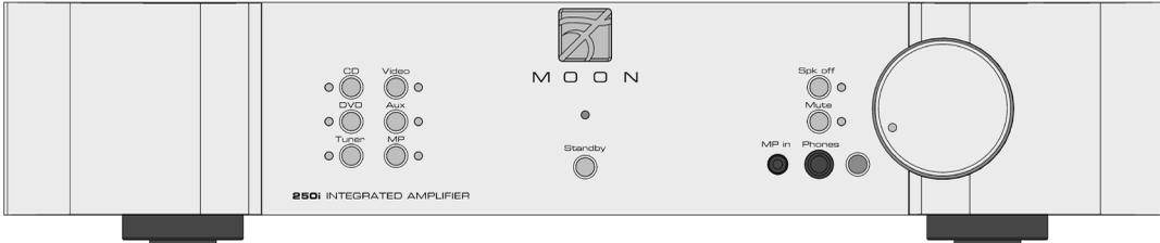
The front panel will look similar to Figure 1 (above). The remote control sensor is located directly to the right of the “Phones” output jack and it should never be blocked, otherwise remote control operation may be compromised.
