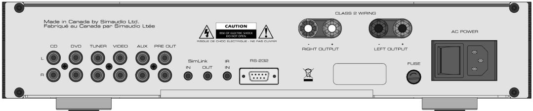
The rear panel will look similar to Figure 2 (above). There are five (5) pairs of single-ended inputs on RCA connectors labeled CD, DVD, TUNER, VIDEO and AUX. The RCA input connectors on the rear panel have been color coded: 'white' for the left channel and 'red' for the right channel.
