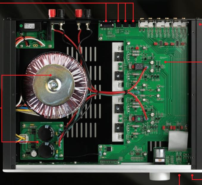
Rigid chassis construction to minimize the effects of external vibrations
