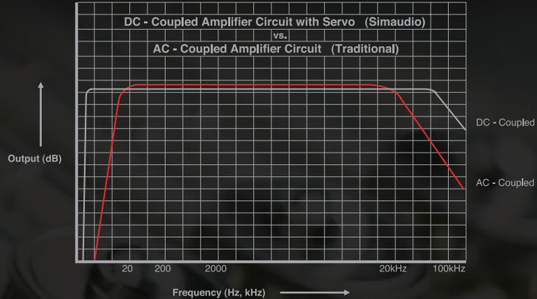
The black frequency response curve in the above figure is virtually flat throughout and beyond the entire audible range as a result of the DC-Coupled circuit employed in the MOON 250i. Conversely, the red frequency response curve of a traditional AC-Coupled amplifier design is far from perfect, both low and high frequencies in the audible range are noticeably diminished:
