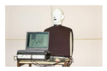
Acoustic dummy with PULSE system to measure airborne sound pressure
