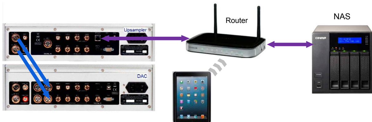
Figure 5 – Using a Vivaldi Upsampler and DAC with a NAS
