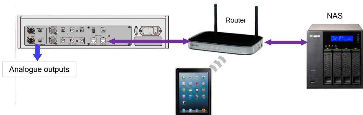
Figure 2 – Using a Rossini DAC with a NAS
