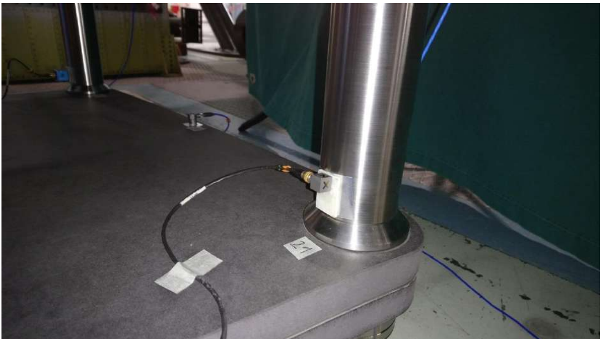
Figure 6. Golia rack during modal tests – Point 21.
