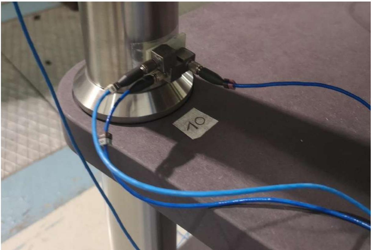
Figure 5. Golia rack during modal tests – Point 10.
