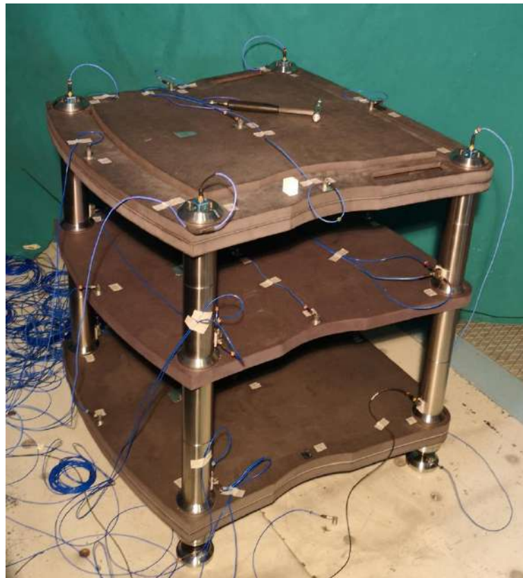
Figure 3. Golia rack during modal tests.
