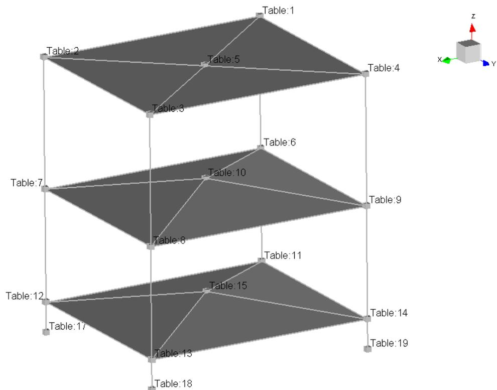
**Figure 2. "Revolution X" wireframe for modal tests.**
