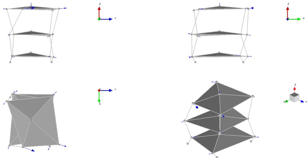
Figure 22. "Revolution X" – Mode 7 – Loaded configuration.
