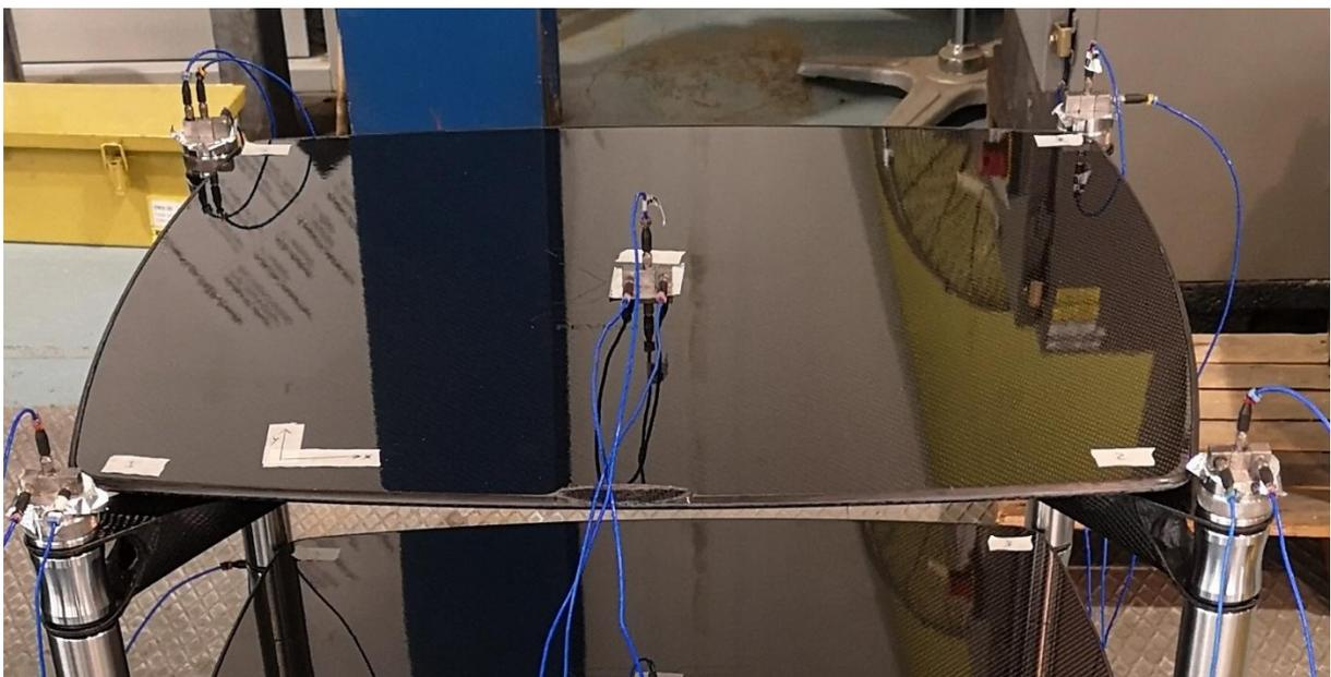
**Figure 4. "Revolution X" – Sensor installation on the top shelf during modal tests.**
