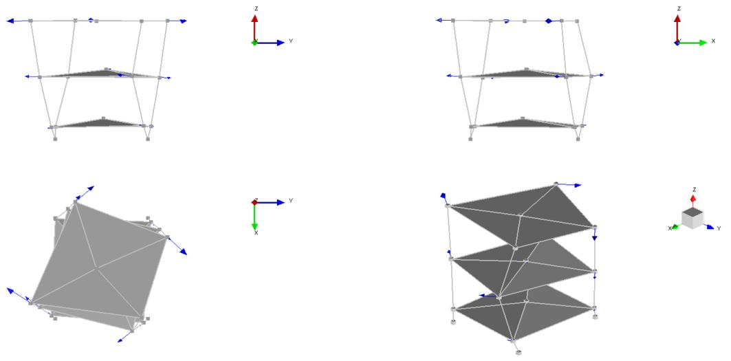
Figure 18. "Revolution X" – Mode 3 – Loaded configuration.
