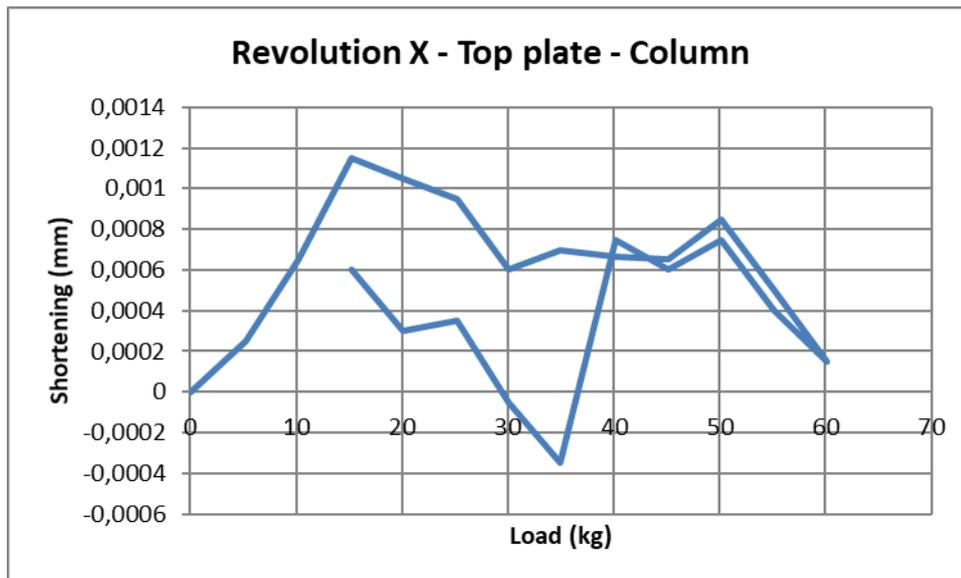
Figure 28. "Revolution X", test 1 – Shortening of corner point as function of applied load.
