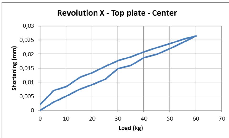
Figure 27. "Revolution X", test 1 – Shortening of central point as function of applied load.
