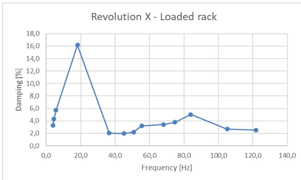
**Figure 15. "Revolution X" – Damping vs. frequency – Loaded rack.**
