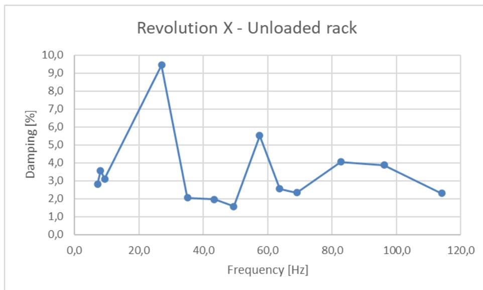
**Figure 6. "Revolution X" – Damping vs. frequency – Unloaded rack.**
