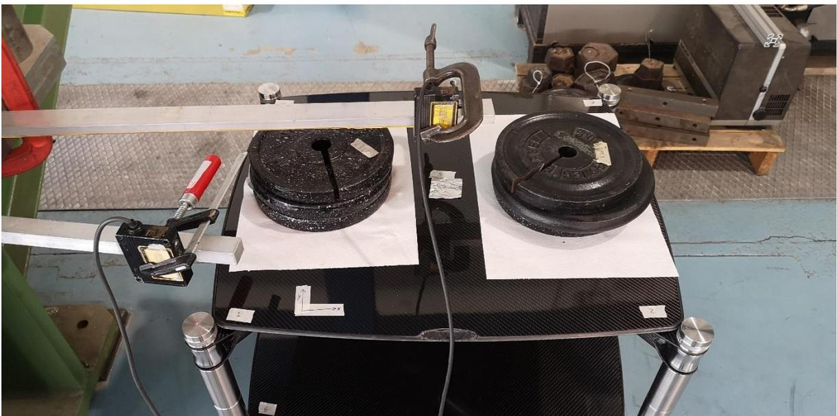
Figure 25. "Revolution X" during static tests – Top shelf loading – Zoom.
