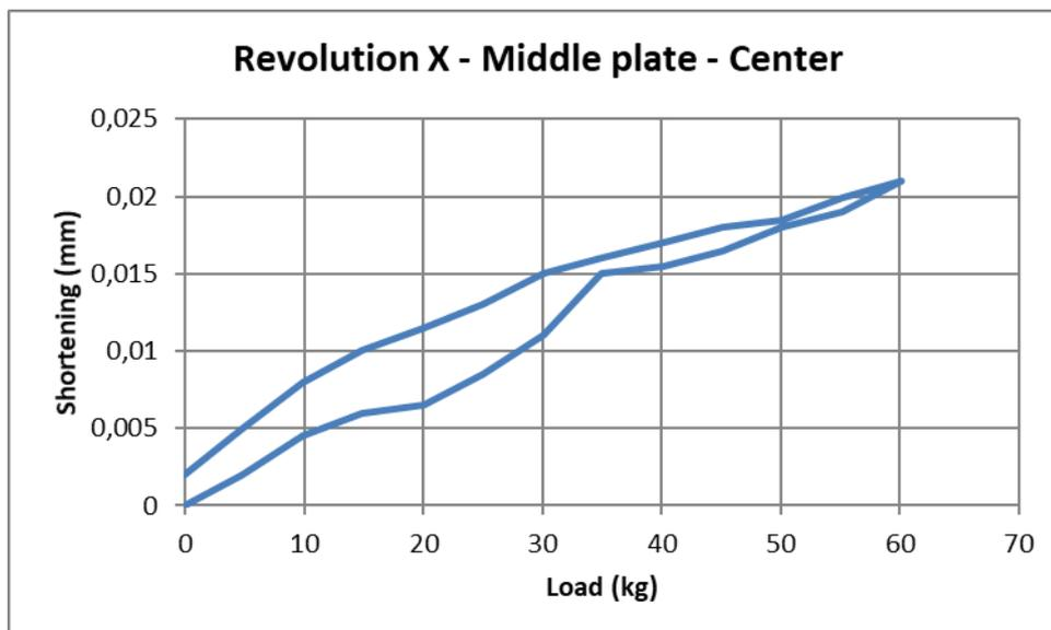
Figure 29. "Revolution X", test 2 – Shortening of central point as function of applied load.
