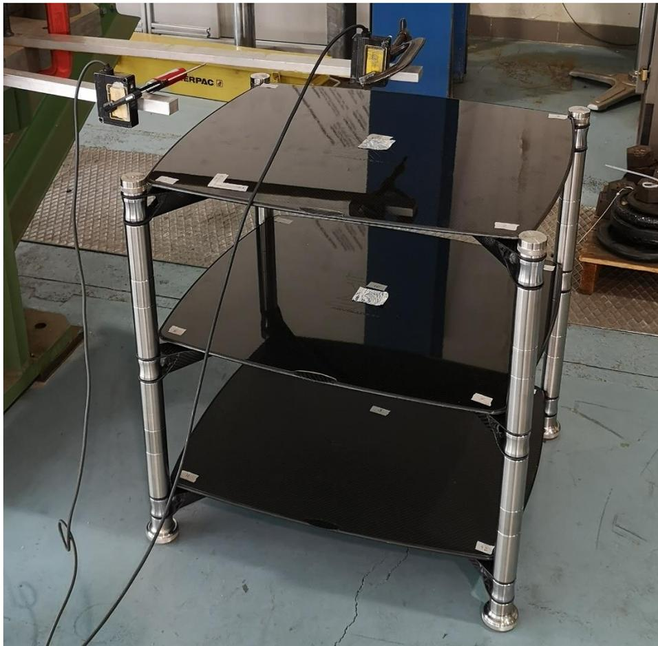
Figure 23. "Revolution X" during static tests – Top shelf loading configuration.
