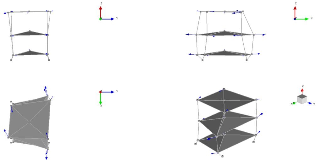
Figure 13. "Revolution X" – Mode 7 – Unloaded rack.
