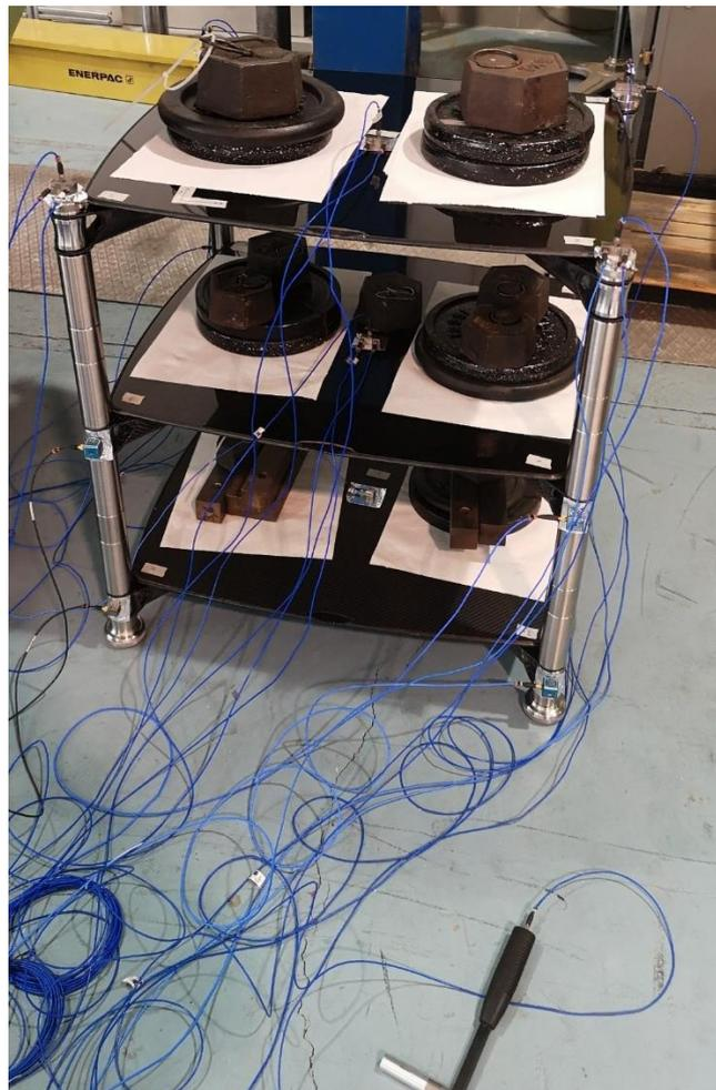
Figure 14. "Revolution X" - Modal tests in loaded configuration.
