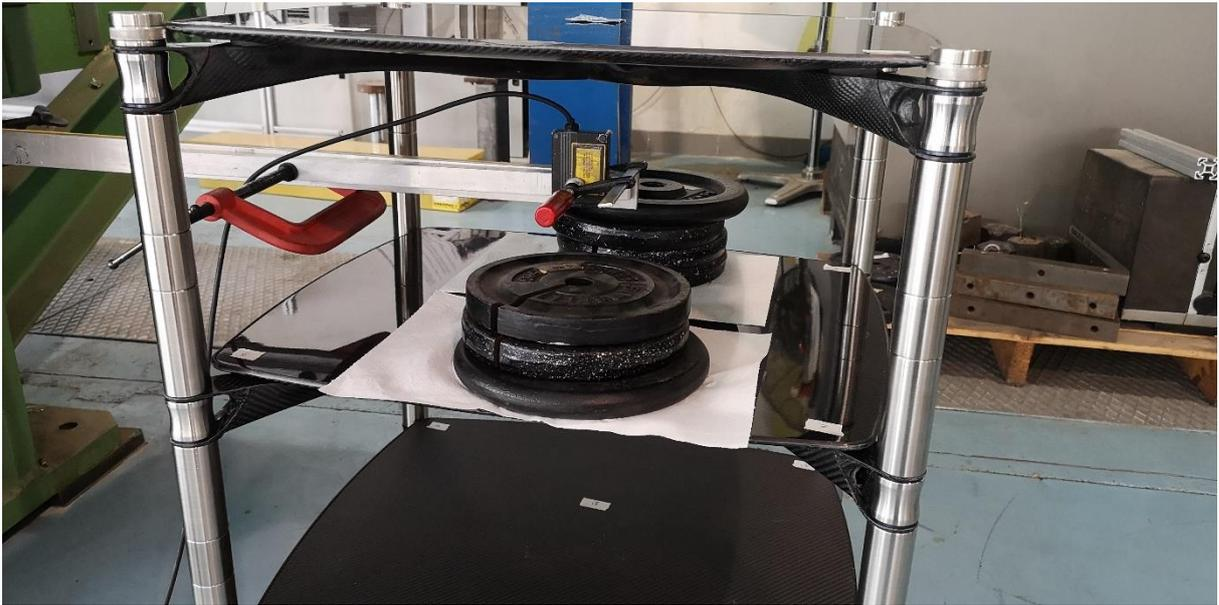
Figure 26. "Revolution X" during static tests – Middle shelf loading.
