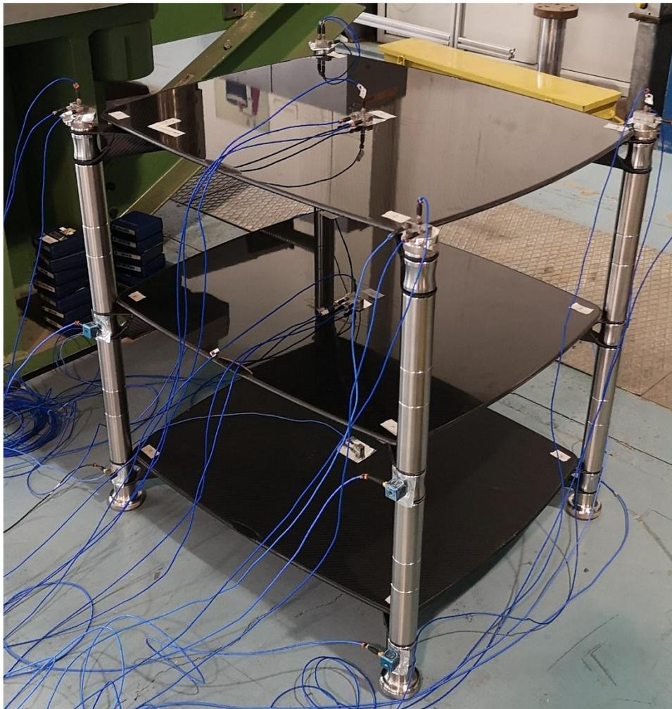
**Figure 3. "Revolution X" during modal tests.**
