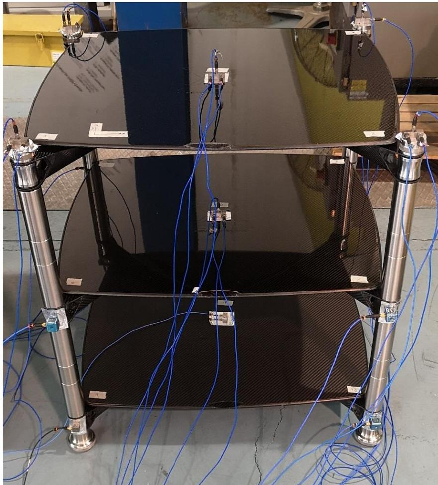
**Figure 5. "Revolution X" –Modal tests in unloaded configuration.**
