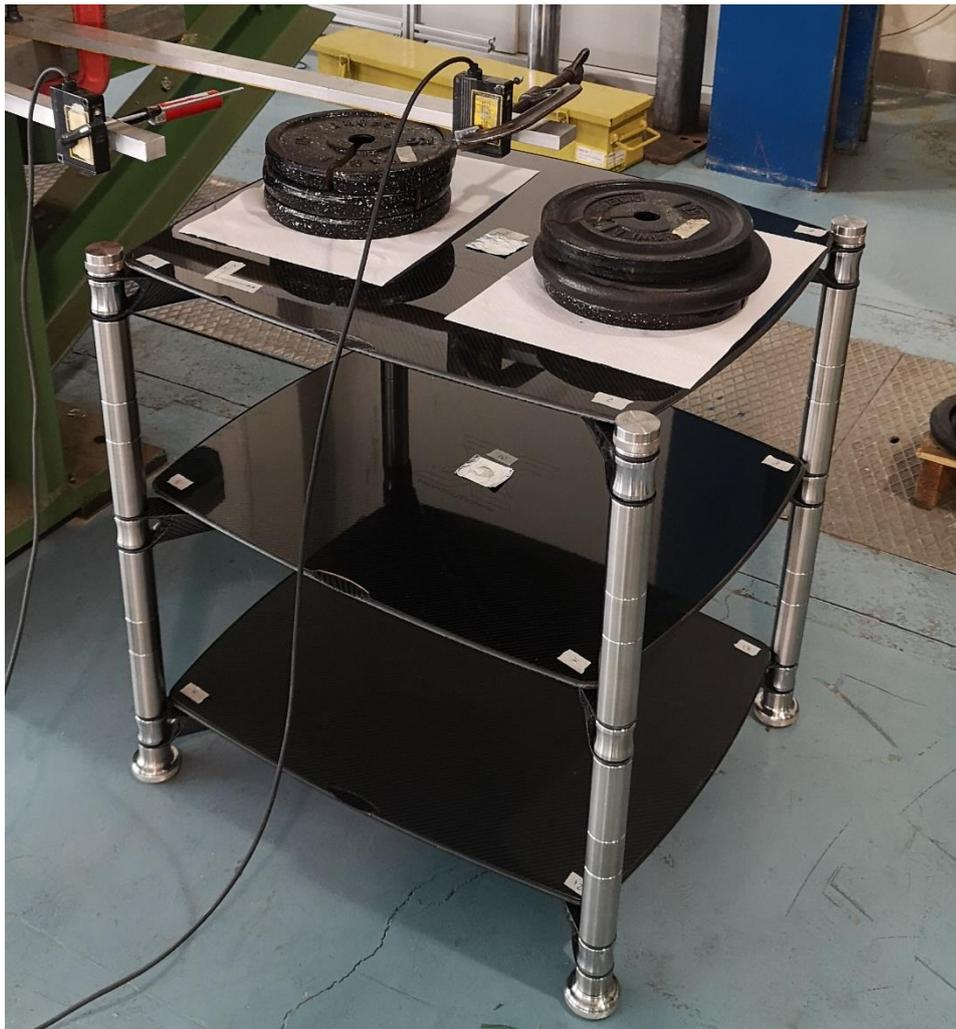
Figure 24. "Revolution X" during static tests – Top shelf loading.
