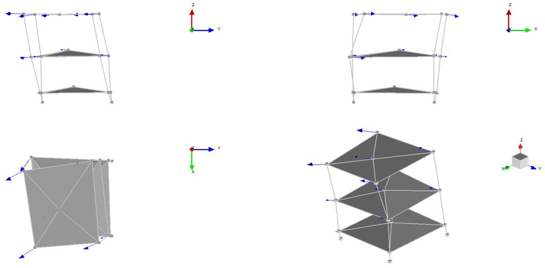
Figure 16. "Revolution X" – Mode 1 – Loaded configuration.
