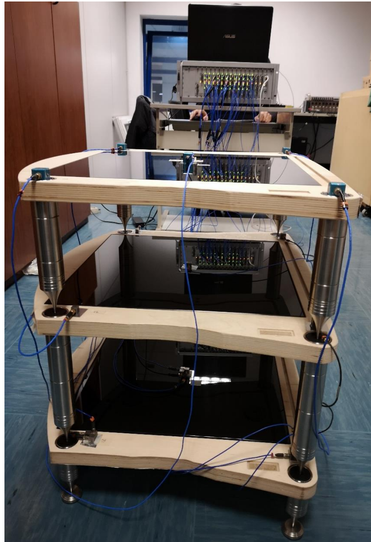
Figure 3. Reference line rack during modal tests.
