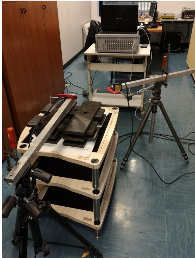
Figure 18. Reference line during static tests – Top shelf loading.
