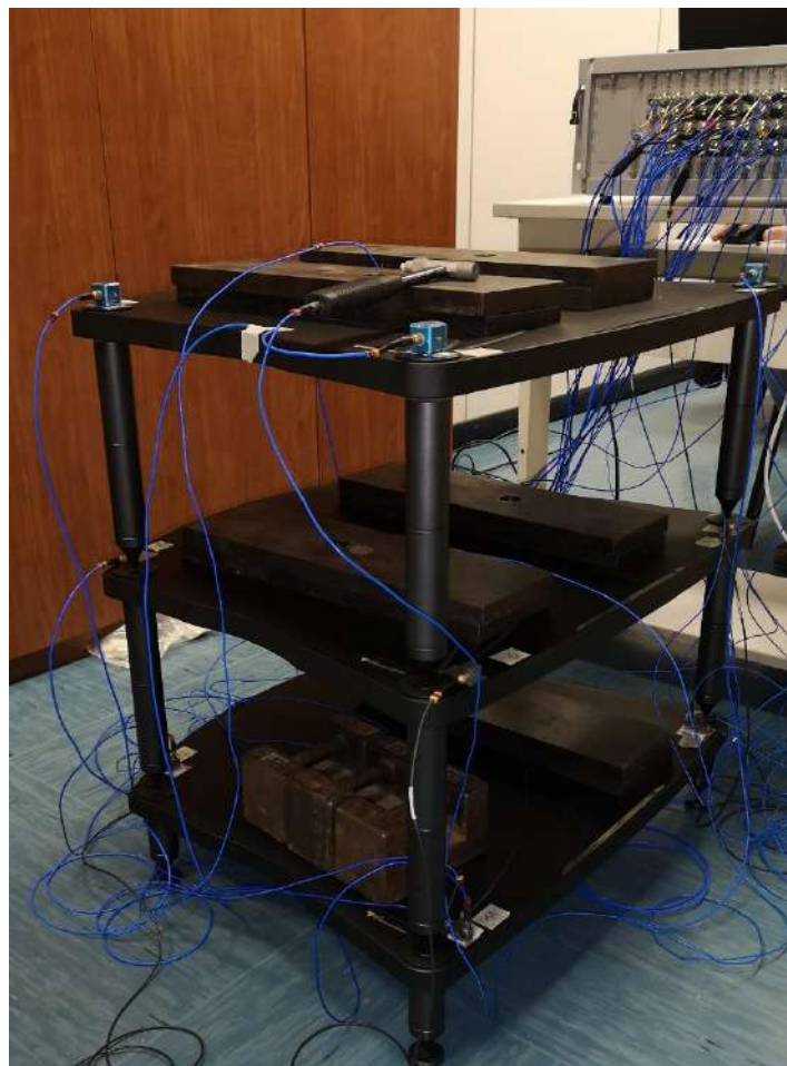
Figure 12. Classic line loaded rack during modal tests.
