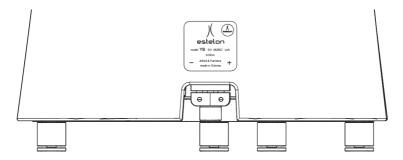
For better result we recommend connecting cables with spades. Loosen the knob, insert the both spades, then tighten the knob.
