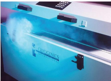
Shunyata Research operates its own onsite *Cryogenics International* computer-controlled cryogenic plant. Liquid nitrogen is used to reduce the temperature of the contents to -320 degrees Fahrenheit. The computer monitors and lowers the temperature by a single degree at a time to prevent thermal shock.
