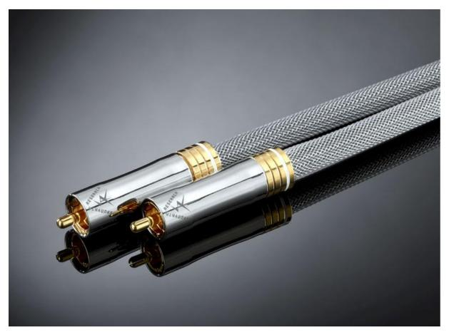
The Venom interconnects come in the same velvet bags as the speaker cables and are quite attractive and flexible. They are built from 16AWG pure OHNO Continuous Cast Copper incorporating Shunyata's exclusive VTX conductor geometry and enclosed in silver-plated OFE, braided shield. The highly polished RCA connectors are 1 1/2" long and require at least 2" clearance behind components for easy connectivity. Balanced interconnects are also available.
