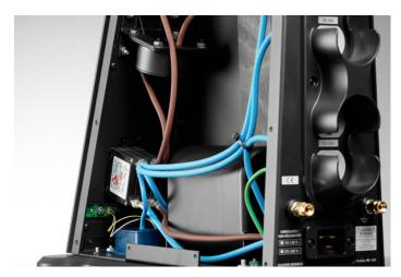
Another feature found on all 3 Denali Series distributors, is a cable cradle support system found on the back of each outlet that prevents AC cords from being pulled out from their weight, especially in the tower Denali designs.
