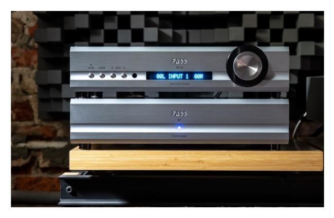
main on/off rocker and self-replaceable fuse, while a 10-pin outlet closer to the center connects it with the preamp via the umbilical cord included in the set.One-box designs house delicate electronics just next to power supplies. The closeness of these bits generates noise, so separating them is the well-
