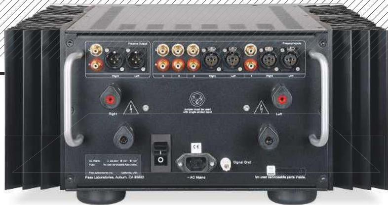
ABOVE: Four line-level inputs are offered, two on both balanced XLR and single-ended RCAs and two on single-ended RCAs only. Balanced and single-ended preamp outs are included alongside superlative binding posts and much-needed handles
