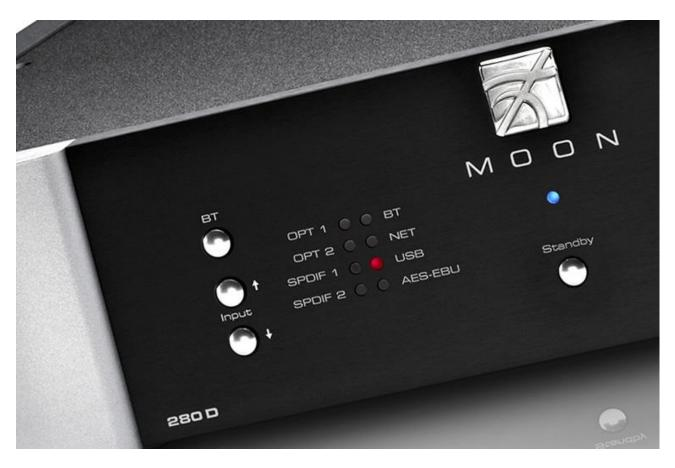
At the faceplate's far left is a column of three silver buttons: the topmost is labeled BT, for Bluetooth discovery mode; the lower two buttons are for scrolling among the various inputs. To the right of these are two columns of four red LEDs each, one for each input: Opt 1 and 2, S/PDIF 1 and 2, BT, Net, USB, AES-EBU.
