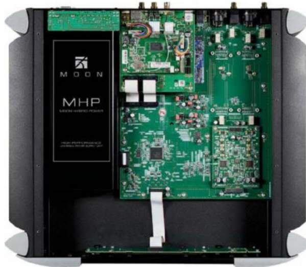
The Moon Hybrid Power (MHP) supply takes up a lot of space inside the 780D.
