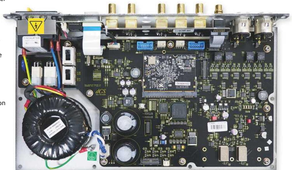
**RIGHT:** Powered by a substantial linear PSU and based on a modified Stream 820 solution, the core upsampling and format conversion is achieved with custom code running on a Spartan-6 processor [centre]
