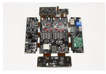
The Lina Master Clock performs the same function as the Rossini Master Clock, and is housed in the smaller Lina chassis. Clocking is used to keep the digital circuits, including power supplies, high-speed signal processing and modulation, in sync with the main audio clock and operating at exactly the same time. This effectively serves to reduce jitter and as a result improves the sound quality when using the network or USB inputs.
