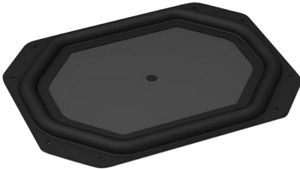
At their simplest it is a speaker driver without the motor structure (magnet, front and back plate and voice coil) mounted in a speaker enclosure along with one or more active drivers. The passive cone reacts to the pressure changes inside the otherwise sealed enclosure created by the active driver. As the active driver moves inward the passive radiator responds by moving outward and vice versa.
